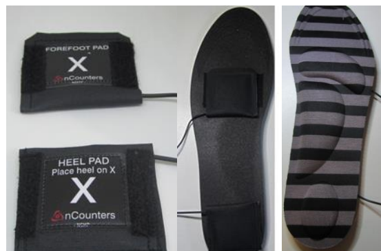
Forefoot and heel sensor pad placement on insole
