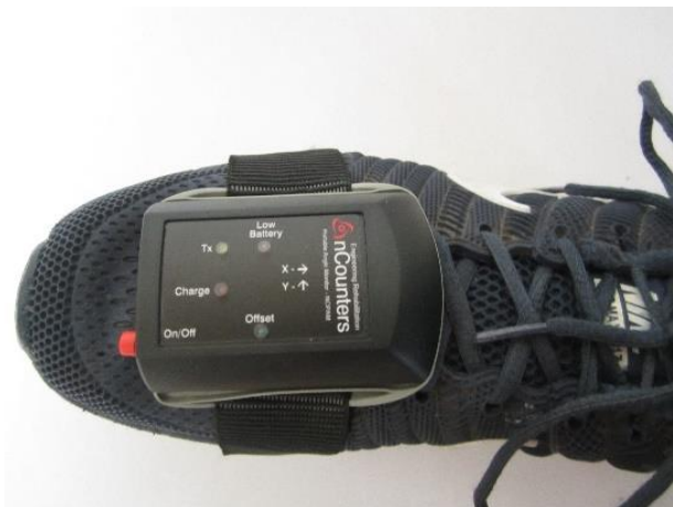
Figure 3 Portable Angle Monitor – in position with the On / Off switch facing away from user's ankle
