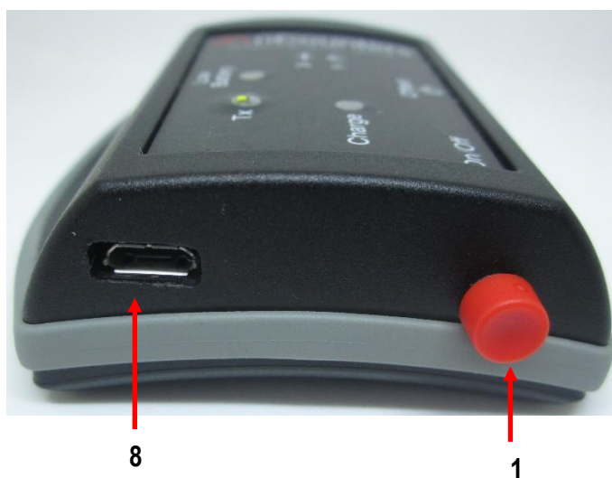
Figure 2 – Portable Angle Monitor – end view. Ensure On / Off switch MUST face away from user's ankle
