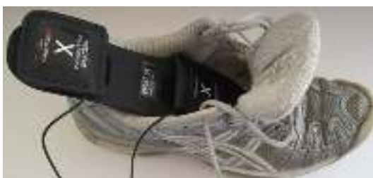
Figure 5: Insert insole with sensor pads into shoe
