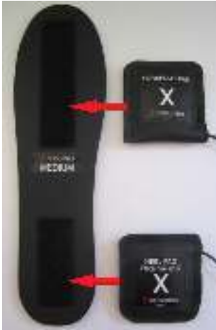
Figure 2: Forefoot and heel sensor pad placement on insole
