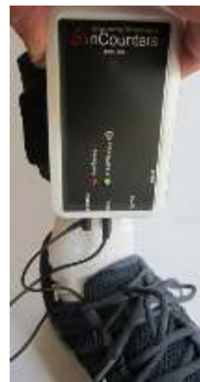
Figure 8: Transmission Tx Load Unit attached to ankle strap
