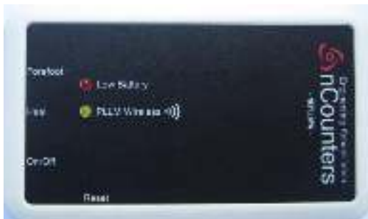
Figure 9: Front wireless Tx Load Unit
