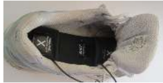
Figure 6: Insole with sensor pads in shoe
