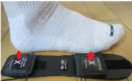
Figure 3: Correct forefoot and heel sensor pad placement
