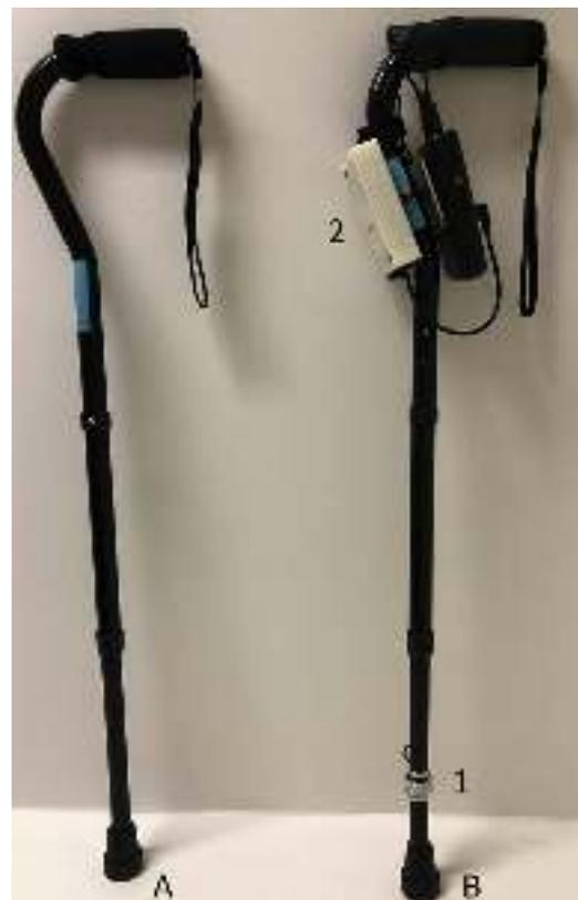
Fig. 1. Study canes. (A) Cane. (B) Instrumented cane with an embedded lightweight uniaxial load cell [1], and data logger [2].
